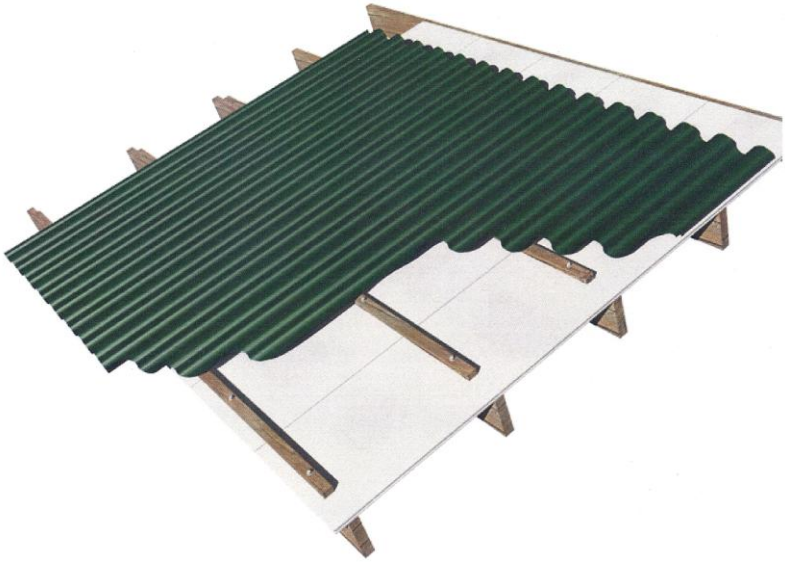
Figure 1: Isoboard® over rafter application with purlins laid directly over rafters
