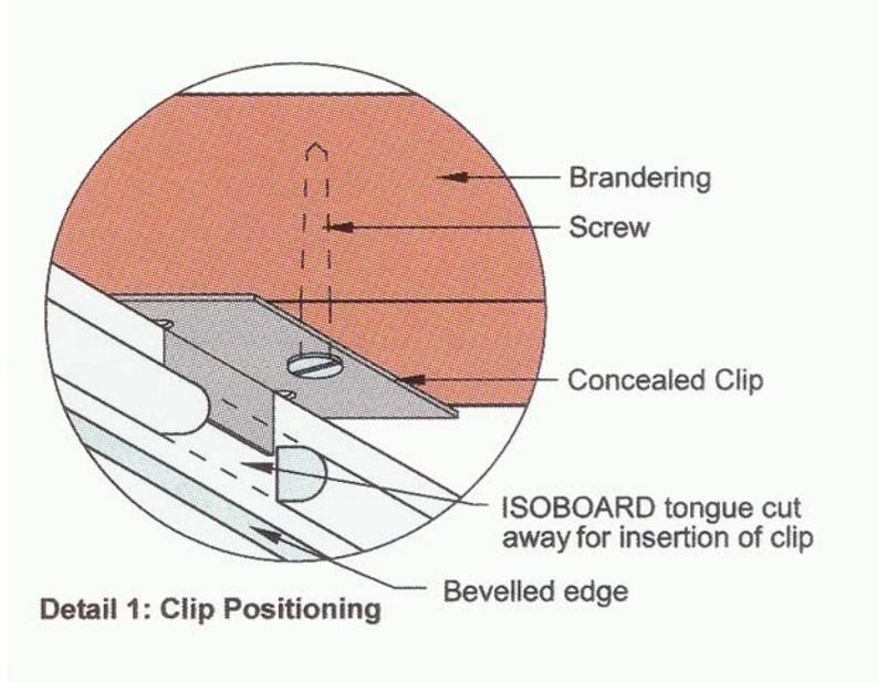
Once the ceiling boards and mechanical fixings have been installed, the boards are pressed against the ceiling supports to ensure thorough contact between the various interfaces.
