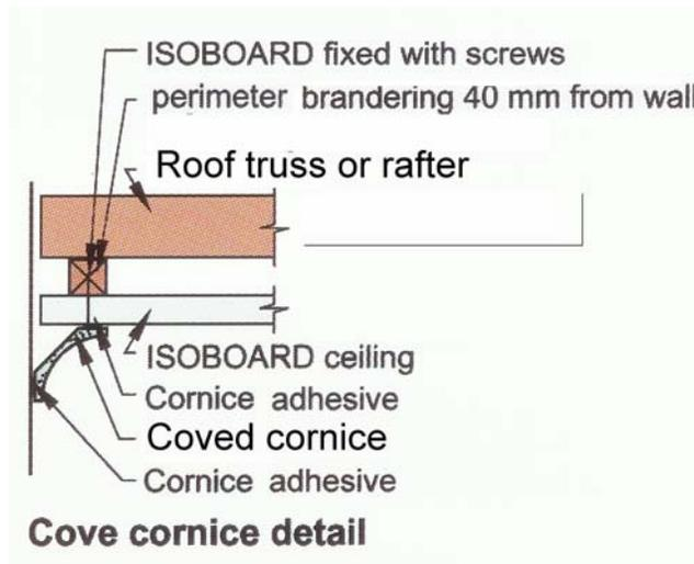
IsoBoard® Nail Up Insulated Ceiling boards are ordered in lengths so as to ensure that butt joints do not occur along the length of ceiling boards. Boards are trimmed to length on site to ensure that once installed a 5 mm gap occurs between the edge or end of the board and the wall.
