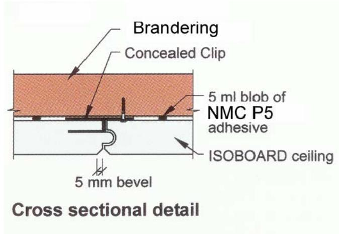
For a flush ceiling effect a flat board is used and after installation the groove formed by the bevelled edge of the board is filled with adhesive, sponged flat and clean and allowed to dry. Thereafter, a PVA/cellulose filler mixture is applied over the joint using a 100 mm wide spatula. Once dry, the length of the joint is sanded smooth with a fine emery paper.
